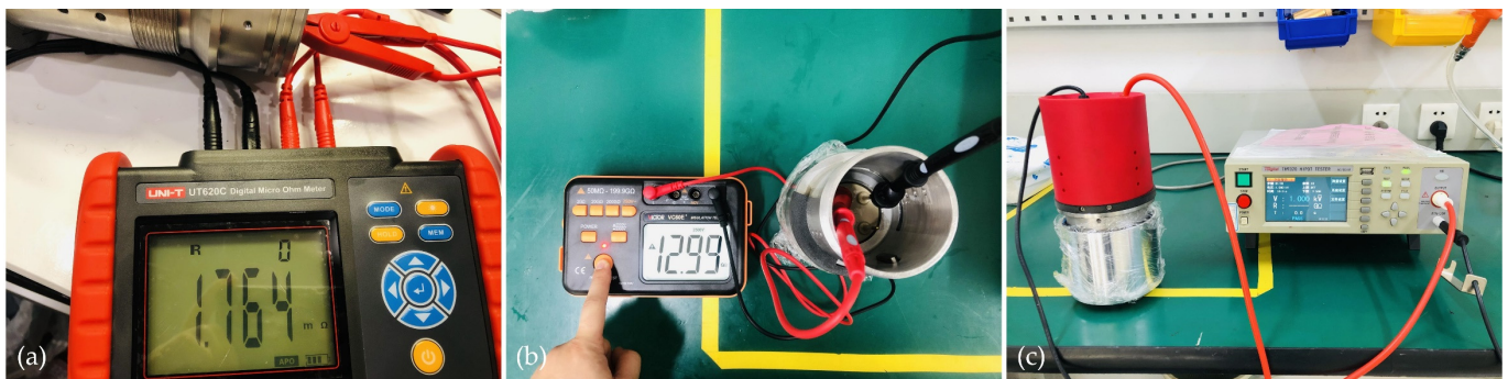
Figure 17. Electrical testing of the prototype: (a) contact resistance test, (b) insulation resistance test, and (c) proof voltage test.
