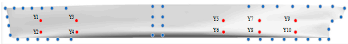
Figure 4. Distributions of variable and fixed points on the Series 60 hull surface (blue: fixed points; red: variable points).
