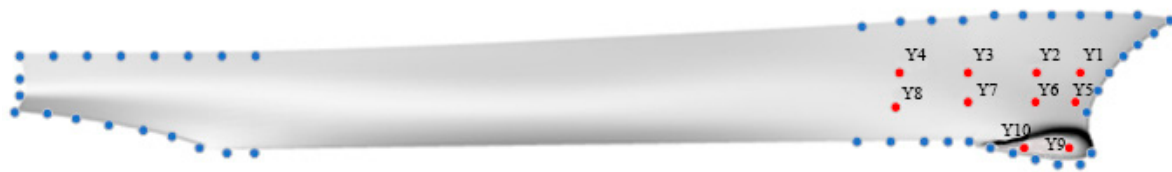
Figure 11. Distributions of variable and fixed points (blue: fixed points; red: variable points).
