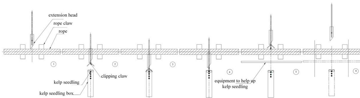
**Figure 5.** Schematic diagram of kelp seedling clipping.
