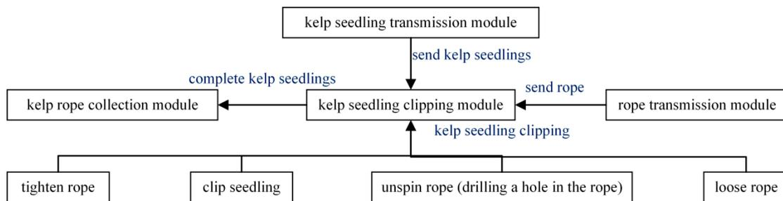
Figure 4. System flow chart for kelp seedling clipping.
