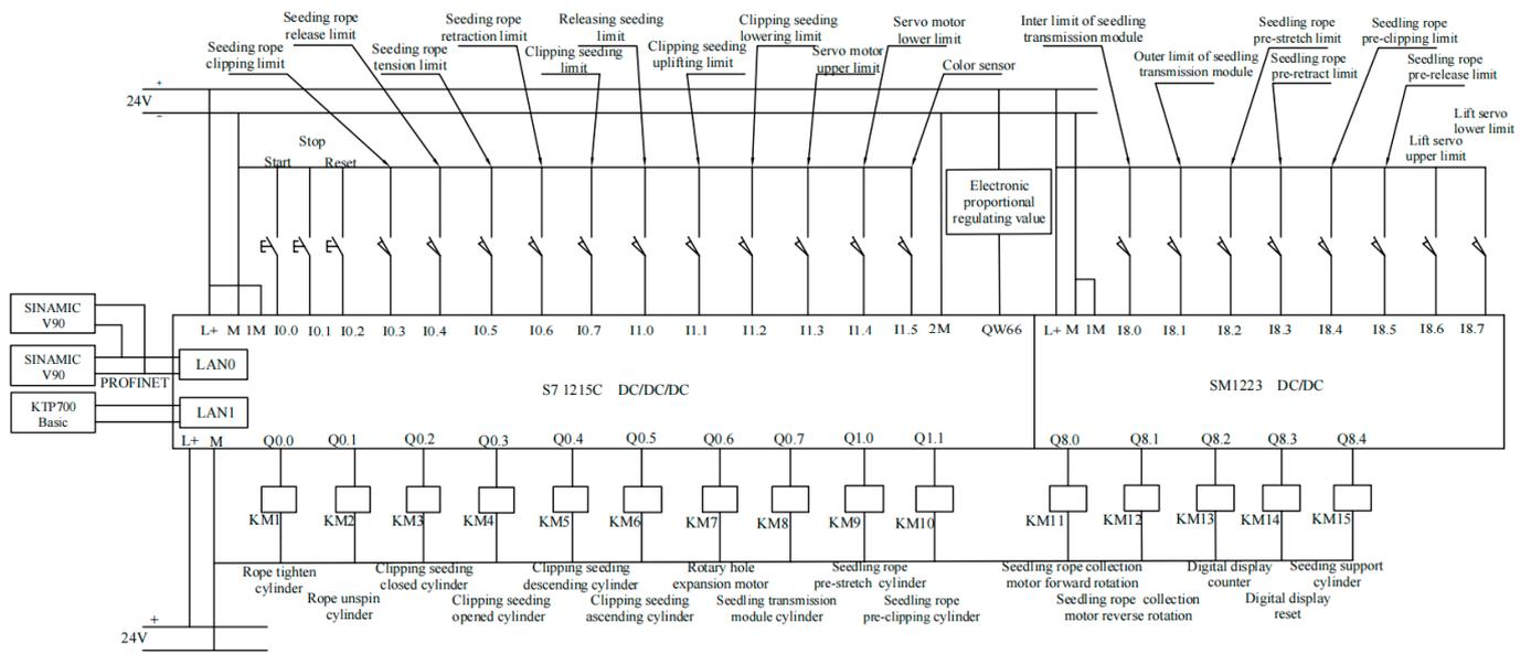
**Figure 6.** Circuit diagram. Note: L+ and M are 24 VDC power inputs, 1 M and 2 M are common terminals, I0.0~I1.5 and I8.0~I8.7 are input button and limit switch, AI0 is analog input, Q0.0~Q1.1 and Q8.0~Q8.4 are control outputs, SIEMENS V90 is a Siemens V90 inverter, KTP700 Basic is a Siemens KTP series touch screen, LAN0 and LAN1 are Ethernet ports, PROFINET is the communication protocol, and KM1~KM15 are 24 V intermediate relays.
