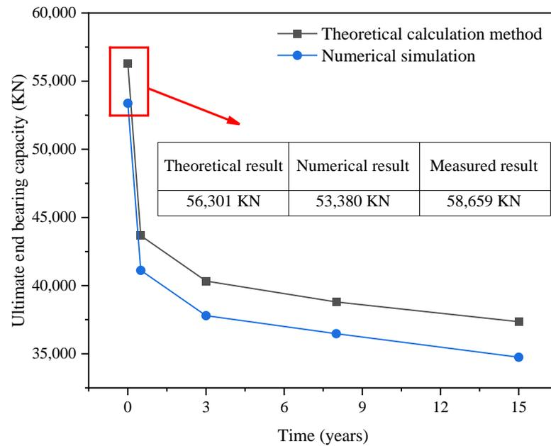
Figure 12. Comparison of the theoretical and numerical results for ultimate end-bearing capacity.
