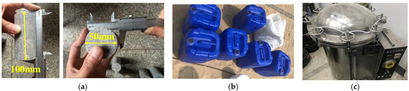
Figure 7. Specimens and equipment for accelerated seawater erosion tests: (a) rock specimens; (b) seawater; (c) deep-water simulation system.
