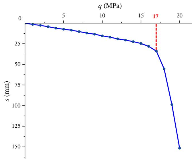
Figure 11. *q-s* curve for test pile obtained by numerical simulation.
