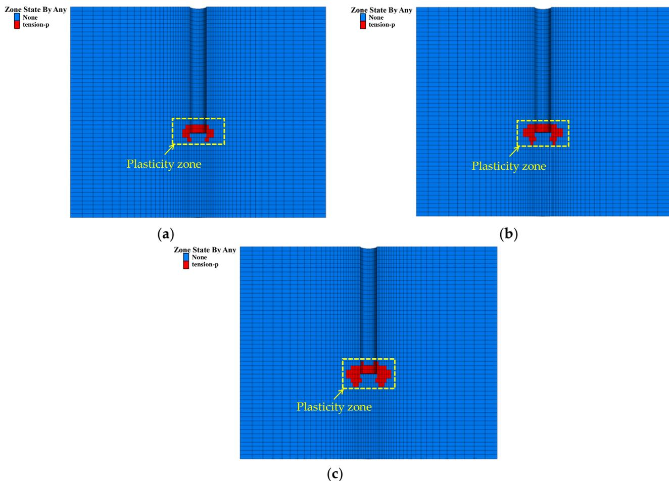
**Figure 13.** Plasticity zones of offshore wind monopile foundations at different times, where the monopile diameter is 2 m, the permeable layer is 12 m, and the rock-socketed depth is 3 m: (a) original stage; (b) after 8 years; (c) after 15 years.
