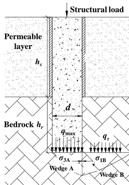
Figure 9. Overall sliding failure pattern of rock mass at the end of the monopile foundation [5,39,40].
