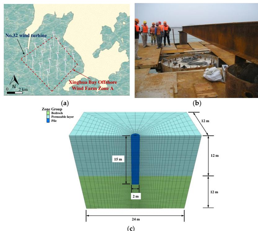
**Figure 10.** Site location and illustration of site test piles and the numerical model: (a) map of the location of the offshore wind farm; (b) test pile for in situ tests; (c) three-dimensional numerical simulation model.
