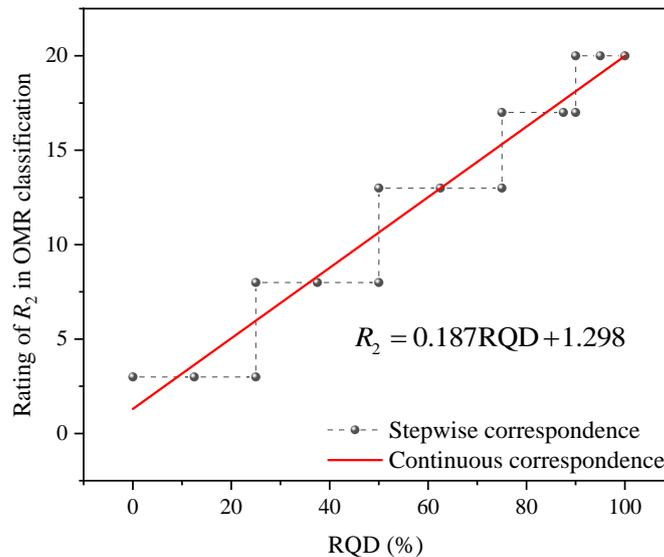
**Figure 4.** Continuity modification of the ratings of the structural integrity of rock mass,  $R_2$ , in OMR classification.
