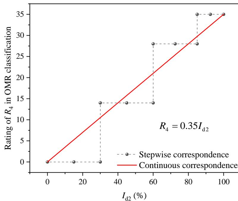
Figure 5. Continuity modification of the ratings of intact rock alterability,  $R_4$ , in OMR classification.
