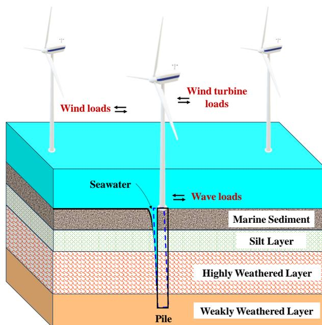
**Figure 1.** Schematic diagram of seawater erosion of the rock around a monopile foundation in the operation phase.
