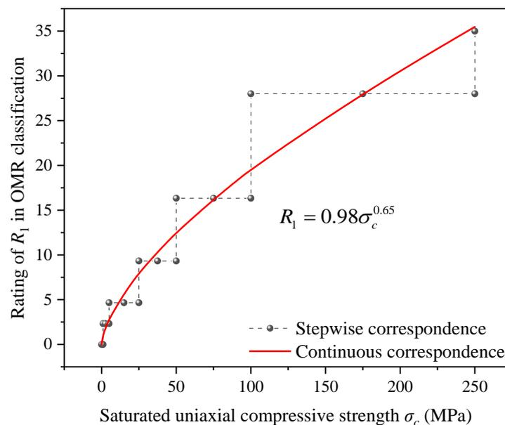
**Figure 3.** Continuity modification of the ratings of the strength of intact rock,  $R_1$ , in OMR classification.
