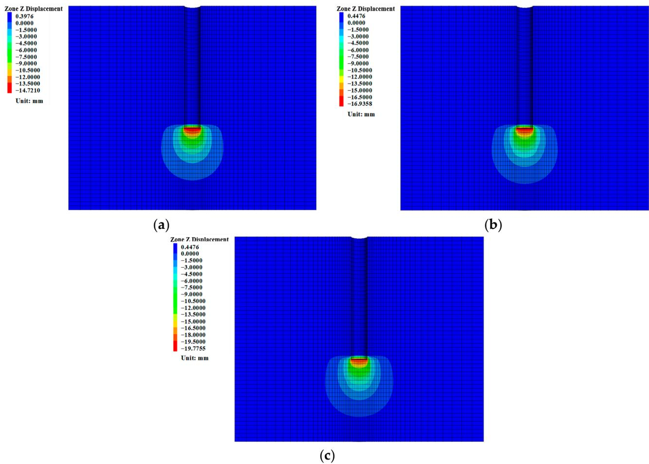
**Figure 14.** Displacements of offshore wind monopile foundations at different times, where the monopile diameter is 2 m, the permeable layer is 12 m, and the rock-socketed depth is 3 m: (a) original stage; (b) after 8 years; (c) after 15 years.
