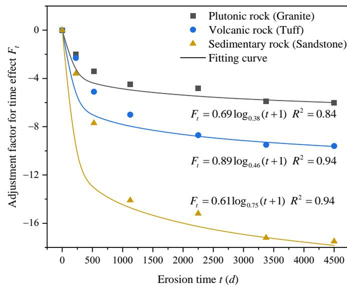
**Figure 8.** Quantitative correlations between the adjustment factor for the effect of time,  $F_t$ , and erosion time,  $t$ , for three rock types.
