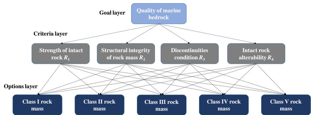
Figure 2. AHP structure for determining OMR classification weights.
