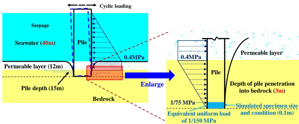
Figure 6. Schematic diagram of the force on marine bedrock for offshore wind monopile foundations.
