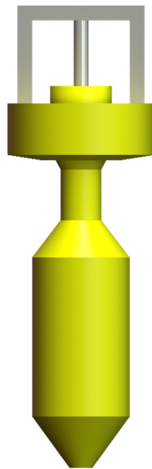
Figure 1. Generic SRPA WEC modeled after a design studied by [27].
