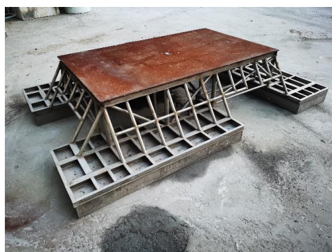
Figure 1. Model of steel framework structure.
