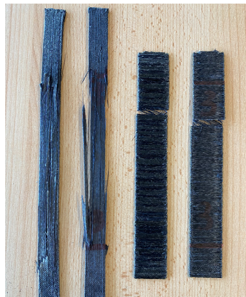
Figure 14. Tensile failure modes of continuous FRP, 0^\circ (left); tensile failure modes of continuous FRP, 90^\circ (right).
