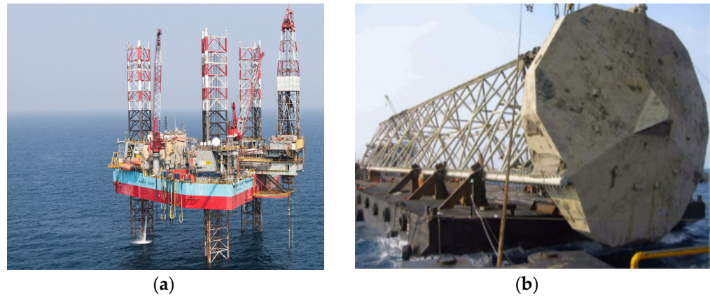
Figure 1. Jack-up drilling rig: (a) jack-up drilling rigs ( https://ramboll.com/projects , accessed on 1 January 2023); (b) spudcan [1].
