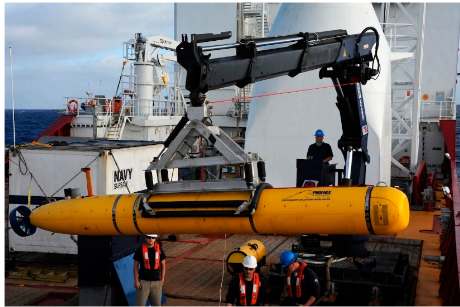
Figure 1. The propeller and control surfaces of unmanned underwater vehicles [5] generally utilize DC motors [6] like those depicted in Figure 2. Credit: Navy photo by Petty Officer 1st Class Peter D. Blair. Department of Defense photographs and imagery, unless otherwise noted, are in the public domain [7].
