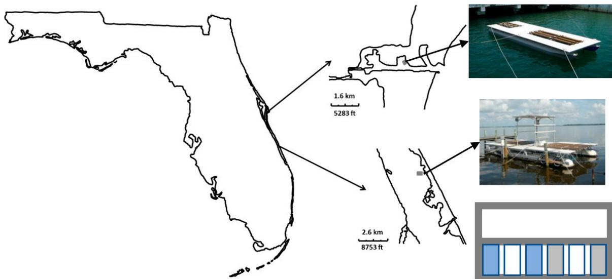
**Figure 1.** Map showing the location of the study sites, the two test barges and a diagram of the frame layout. Panels are suspended horizontally on PVC frames and suspended on the test barges.
