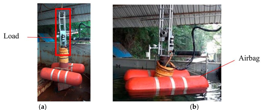
**Figure 14.** Drifting platform setup for the water surface stabilization experiment. (a) Empty water pool, (b) Full water pool.
