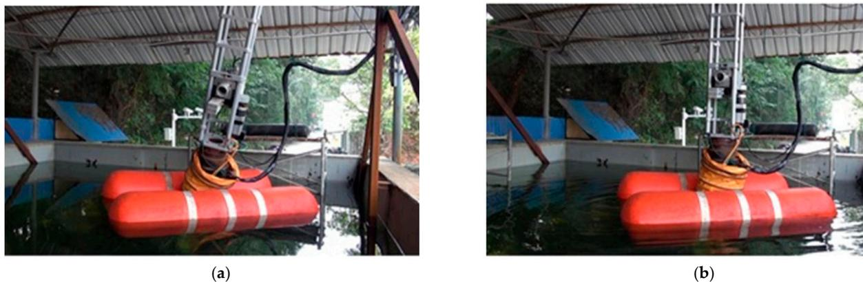
**Figure 15.** Experimental setting of large angle attitude leveling of the drifting platform. (a) Initial status of the drifting platform, (b) Status after leveling of the drifting platform.
