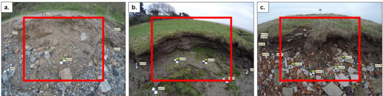
Figure 4. Red squares highlight the estimated central portion of the image where Agisoft Photoscan markers should be placed on GCPs: (a) Thurstaston, (b) Silverdale and (c) Crosby.
