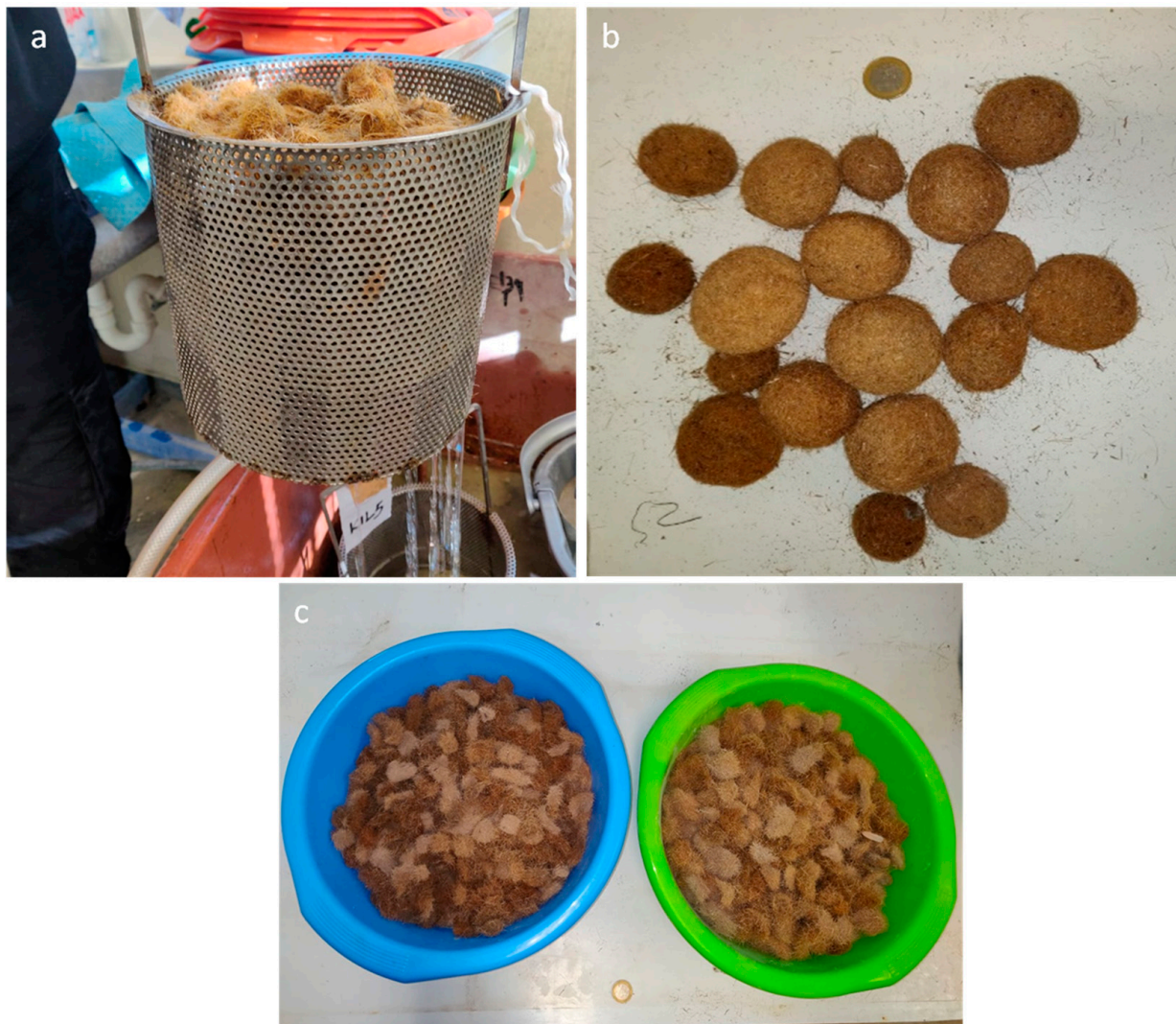
Figure 2. (a,b) Posidonia oceanica and drying ball samples as the raw material, and (c) the samples after washing.
