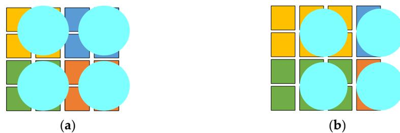
**Figure 7.** Spot distribution under different link misalignments. (a) Small degree of link misalignment. (b) Large degree of link misalignment.
