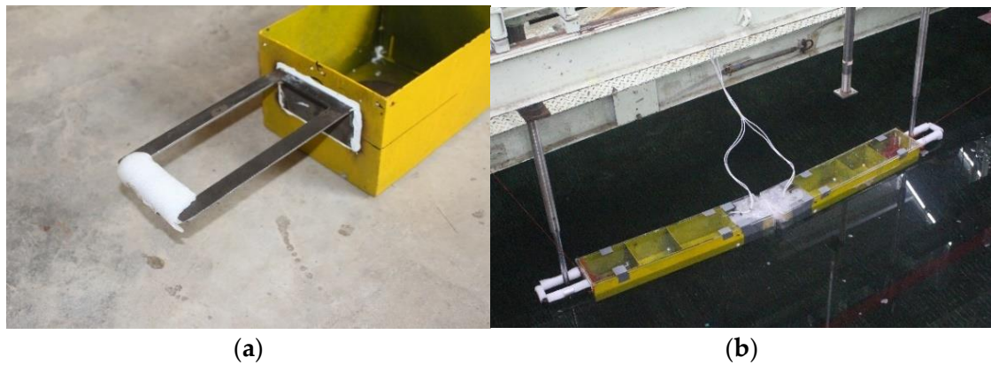
Figure 3. The mooring system and the floating body. (a) The navigation board. (b) The mooring system.
