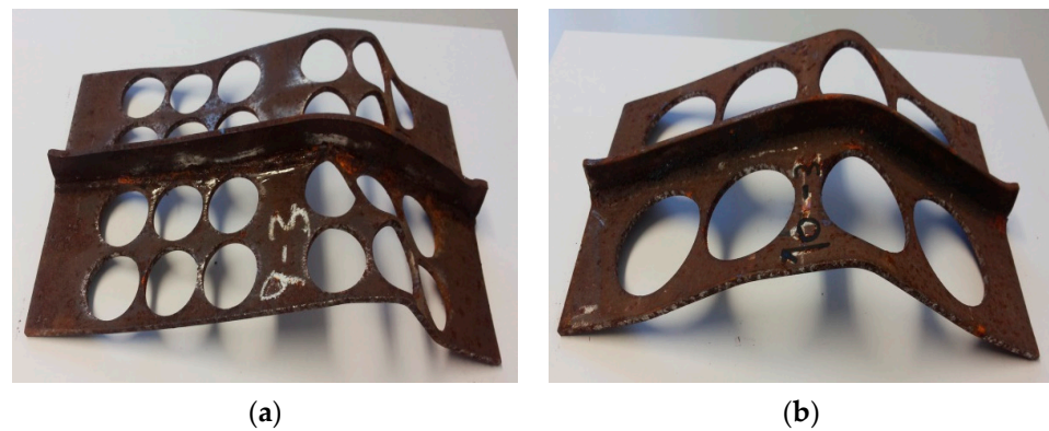
Figure 11. Post-collapse deformed shape for n = 24 , DoO = 42.90\% , SP-NS9-3 (a) and SP-NS10-3, n = 8 (b).
