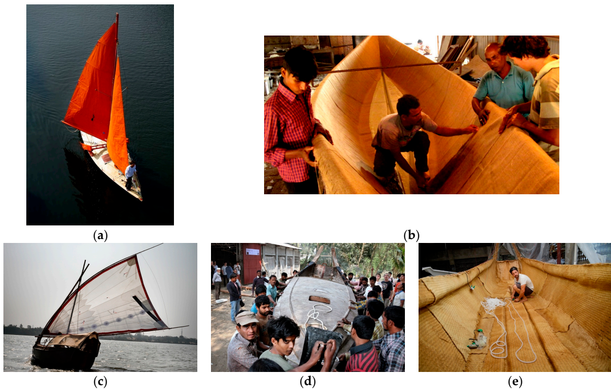
Figure 23. (a) TaraTari, a 9 m long boat built using jute fibers; (b) construction of the TaraTari using local materials; (c) Gold of Bengal, made entirely from jute fibers and polyester matrix; (d) locals in Bangladesh working on the Gold of Bengal boat; (e) low-technology manufacturing processes used for the Gold of Bengal, made entirely from jute fibers and polyester matrix. Photo credits: Corentin de Chatelperron/Gold of Bengal Association.
