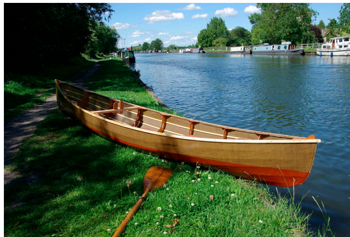
Figure 21. Flaxland canoe, built using flax natural fibers. Photo credit courtesy of Flaxland.
