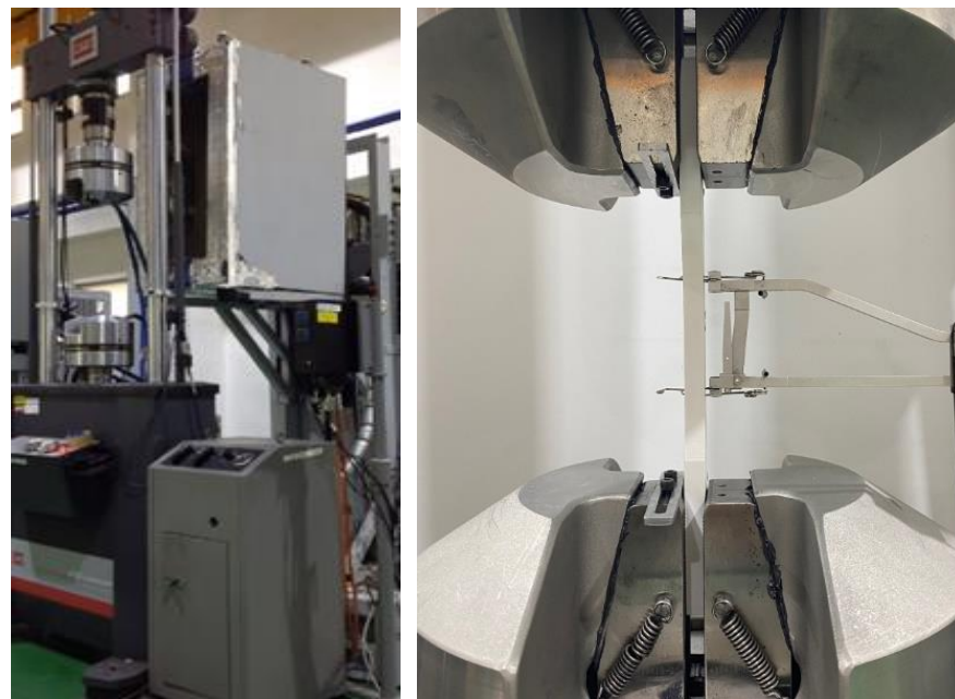
Figure 5. Tensile test machine (left) and test set-up (right) for ABS material.
