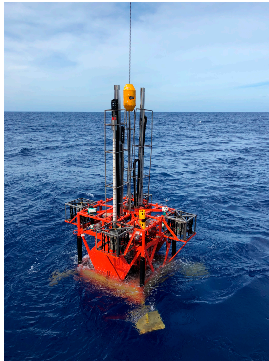
Figure 5. In Situ Surveying Equipment of Engineering Geology in Complex Deep Sea, SEEGeo.
