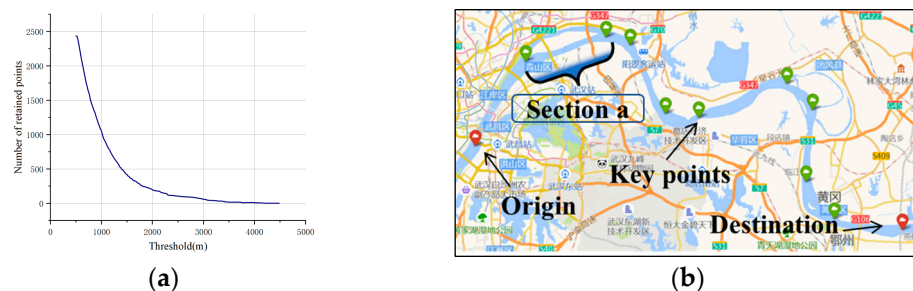
Figure 10. (a) Relationship between distance threshold of DP algorithm and number of retained key points in the channel’s centerline. (b) Visualization of key points.
