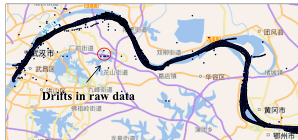
Figure 7. Raw AIS data covering an area of 141 Km of Yangtze River.
