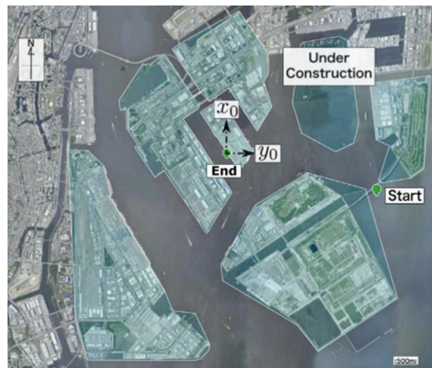
Figure 14. Simulation environment of path planning in the work by [35]. Polygons with white lines represent the obstacles in harbor environment.
