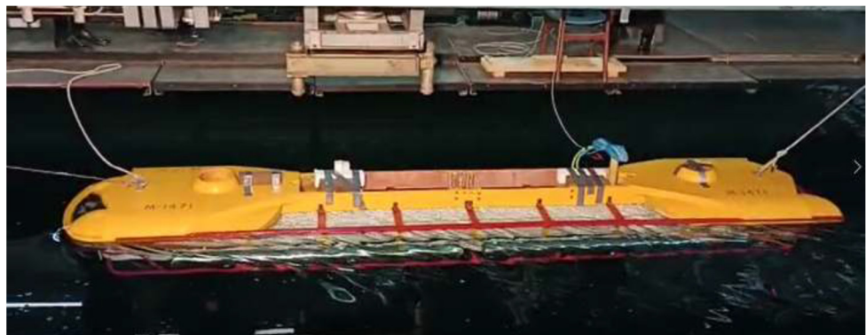
Figure 6. Towing test in calm water.
