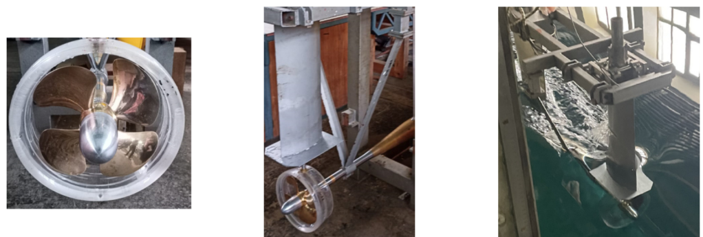
Figure 9. Propeller in the nozzle (left); setting of the equipment (middle); and open water test (right).
