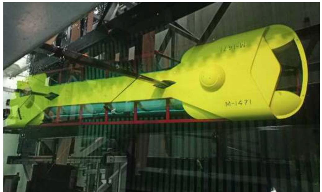
Figure 4. Submarine model mounted on sabre-shaped girders and installed under the carriage for resistance tests in deepwater conditions.
