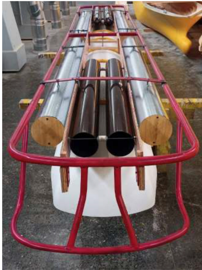
Figure 2. Bottom view of the submarine model (lower half of the pressure hull, battery pods, variable ballast tanks, and lower exostructure).
