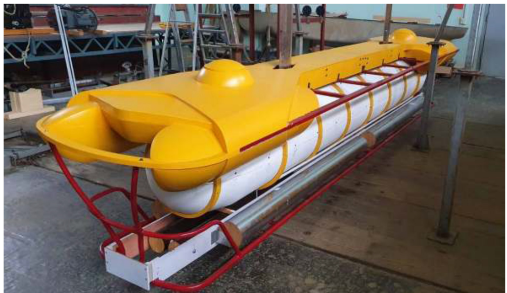
Figure 3. Submarine model (front ISO view) completed for tests in deep water.
