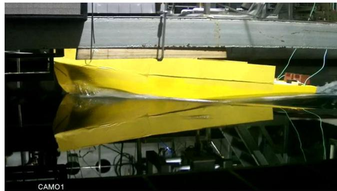
Figure 8. Typical sailing condition of the model (speed 12.4 kn).
