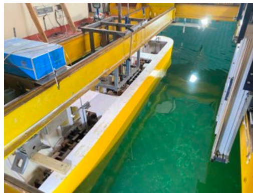
Figure 2. Resistance tests in towing tank.
