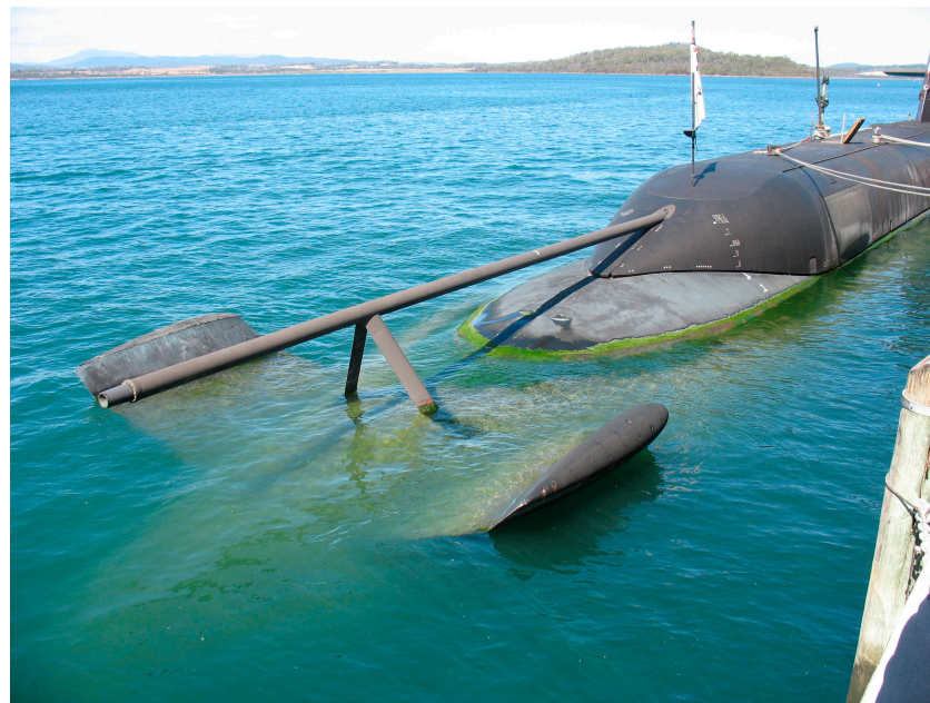
Figure 2. Example of submarine showing fouling over the lower portion of the hull.
