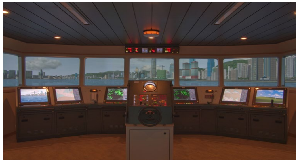
Figure 12. Full-mission ship-handling simulator of the Korea Institute of Maritime and Fisheries Technology.
