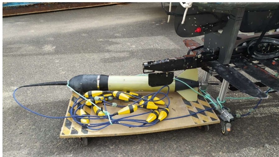
Figure 2. The recording system used with the Waveglider ® ™ Sv2 (Pambuoy system).
