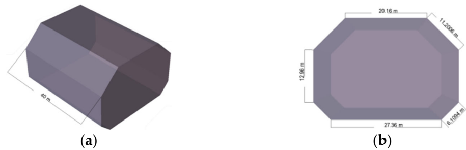
Figure 6. View of the (a) 3D model and (b) dimensions of the prismatic storage tank of the FLNG vessel drawn with SeSam GeniE software (manager V6.1-02).
