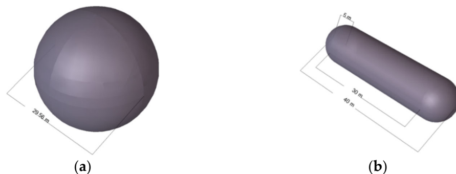
Figure 8. Dimensions of (a) spherical storage tank and (b) cylindrical storage tank of the FLNG vessel obtained using SeSam GeniE software (manager V6.1-02).
