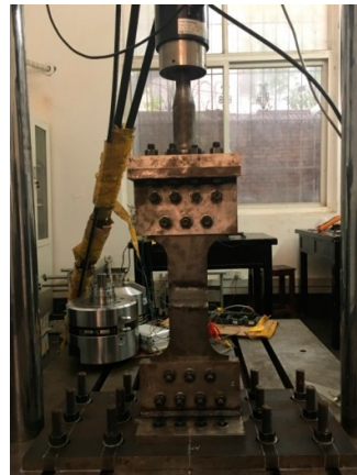
Figure 2. Scheme of fatigue crack growth test.
