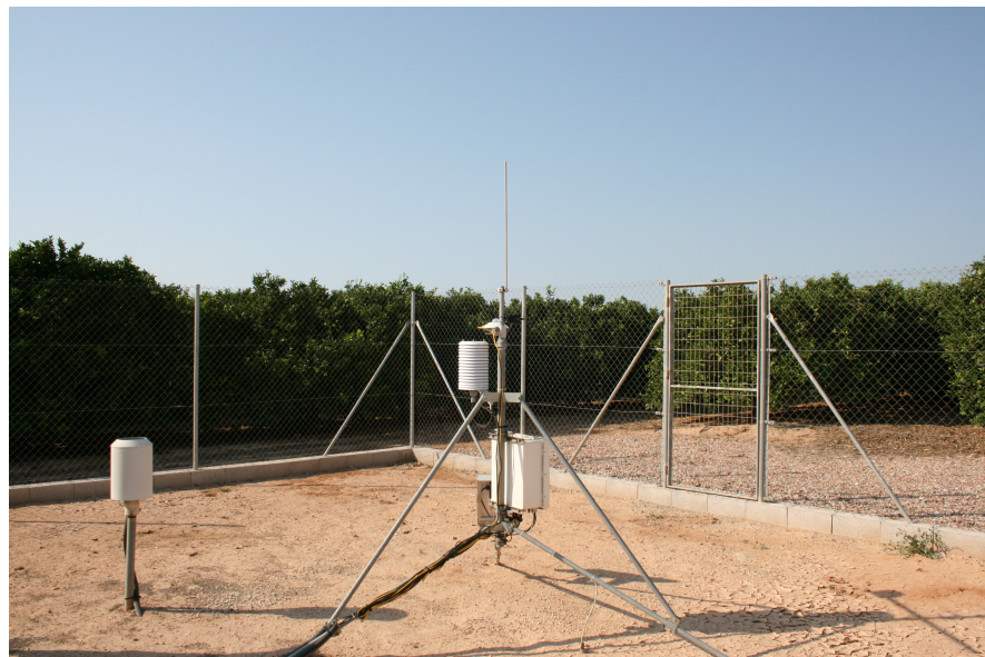
Figure 6. Type of automatic station used to collect agro-climatic information.
