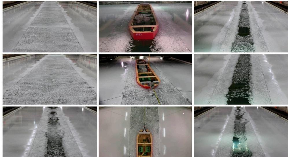
**Figure 3.** Sample images of the real ice channel dataset (images taken from the experiment).
