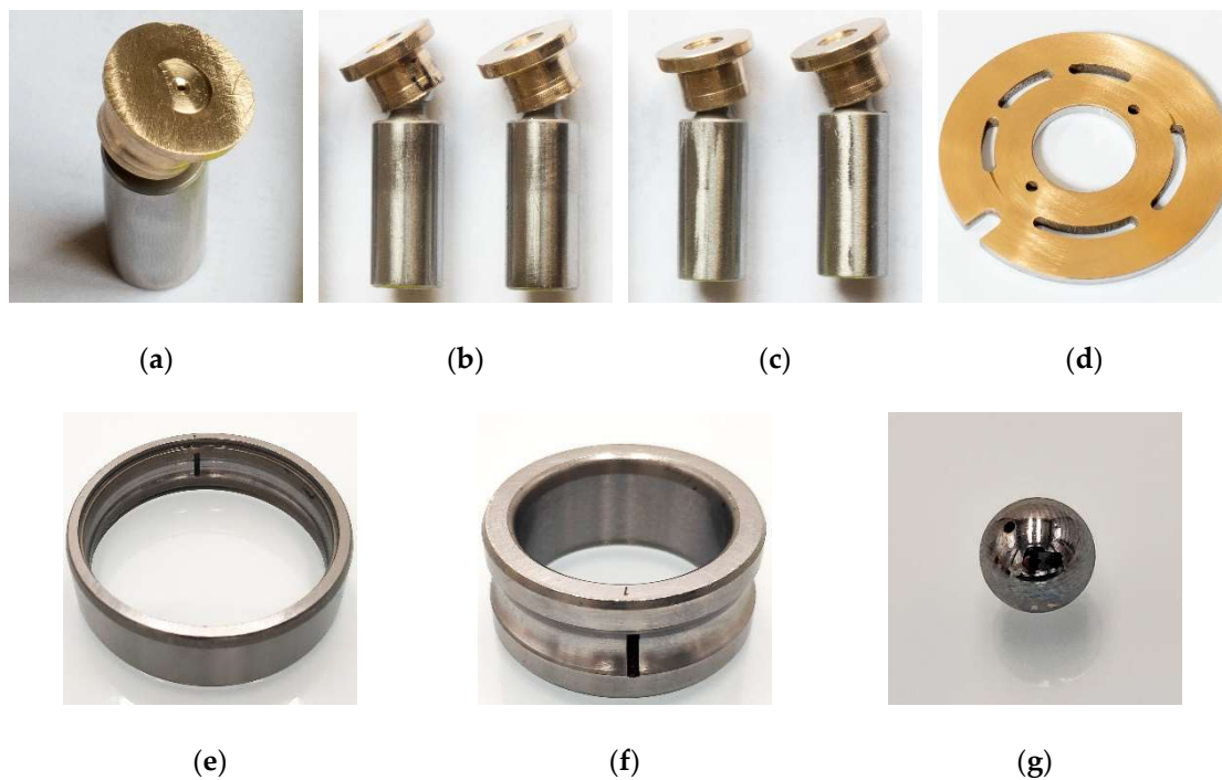
Figure 6. Photographs of various faulty components of plunger pumps used for the testing. (a) Wear of shoe; (b) loose shoe; (c) wear of plunger; (d) wear of port plate; (e) fault of outer ring; (f) fault of inner ring; (g) fault of rolling element.
