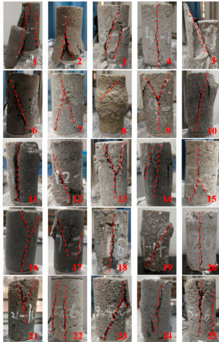
Figure 16. Specimen failure mode.
