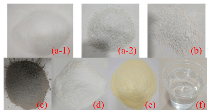
Figure 2. Similar material basic components of rock mass under seepage and dynamic coupling: (a-1) 0.3–0.5 mm quartz sand; (a-2) 1.0–2.0 mm quartz sand; (b) barite powder; (c) cement; (d) sodium silicate; (e) rosin; and (f) glycerin.
