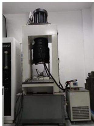
Figure 5. KD-II-type high pressure and low temperature hydrate mechanical properties testing system.
