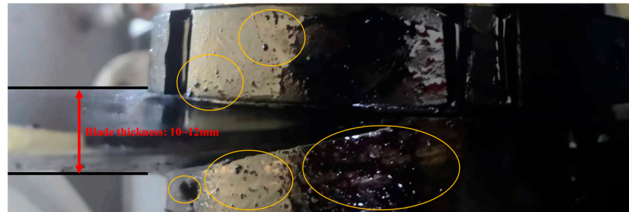
Figure 3. Gravel on the impeller surface.
