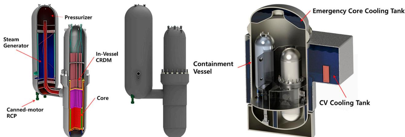
**Figure 4.** Configuration of the safety features of the BANDI-60S SMR to be used in floating nuclear power plants in South Korea, reproduced with permission from Elsevier B.V. 2024 [43].
