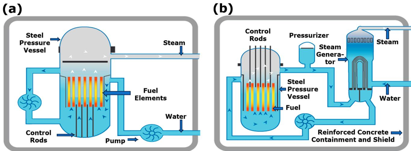
**Figure 3.** Schematics of (a) boiling water reactor (BWR) and (b) pressurized water reactor (PWR), extracted from World Nuclear Association [38].
