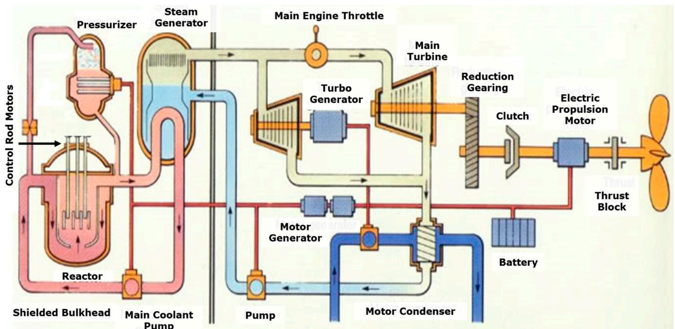
**Figure 1.** Schematic diagram of a typical pressurized water nuclear propulsion system used in a nuclear-powered maritime vessel [7].
