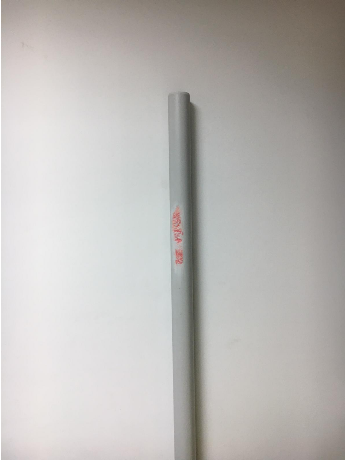
Figure 3. Damaged pipe used in the experiment (red-colored region is defined as “damage”).
