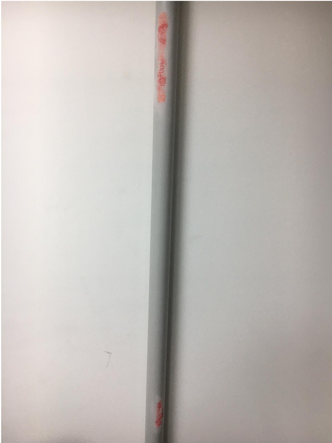
Figure 2. Damaged pipe used in the experiment (red-colored region is defined as “damage”).
