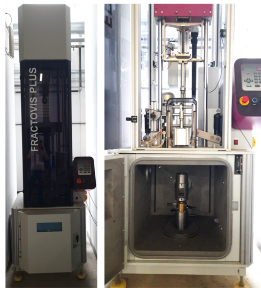
Figure 3. Drop impact test setup.
