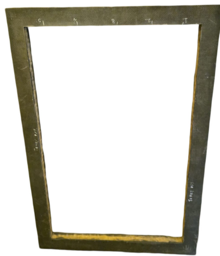
Figure 6. Sandwich panel after cutting the specimens.
