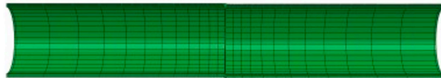
(a) Bi-layer pipe having centerline offset with equal thickness and diameters
