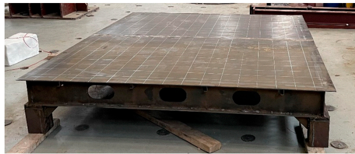
Figure 14. Diagram of the actual plated grillage specimen.
