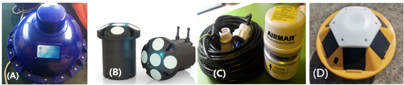
Figure 3. Observation equipment for the drift experiment. (A) Tracking buoy, (B) acoustic Doppler current profiler, (C) multi-parameter weather station, and (D) small wave observation buoy.
