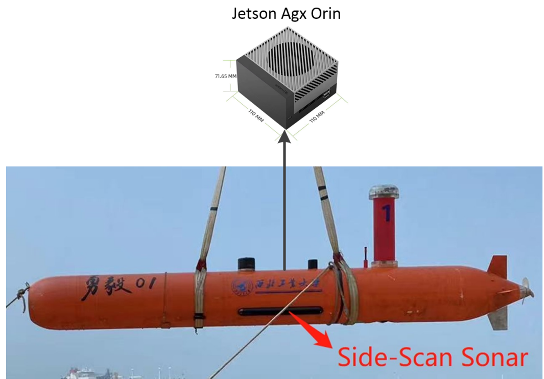
Figure 5. Schematic diagram of embedded processor installation location in AUV.
