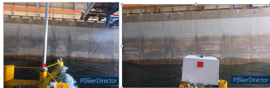
Figure 29. Wave breaking on FOWT and FOSS platform.
