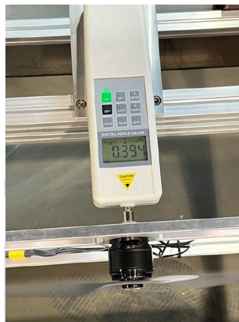
Figure 24. The 50-year return period wind thrust of the wind turbine model measurement diagram.
