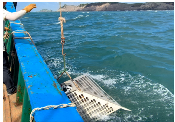
Step2: Deploy the seafloor observation subsystem down towards the destination seabed
