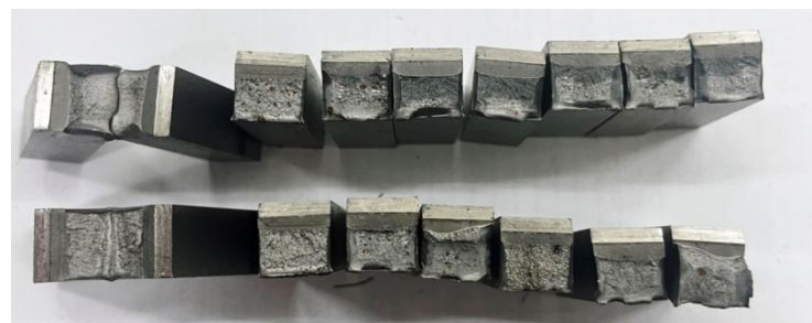
Figure 7. Specimens for dynamic fracture toughness.
