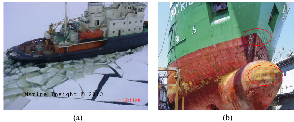
Figure 1. (a) A ship on ice-covered sea and (b) damages to MV Patriot's hull (see the red circles) due to repeated ice floe impacts.
