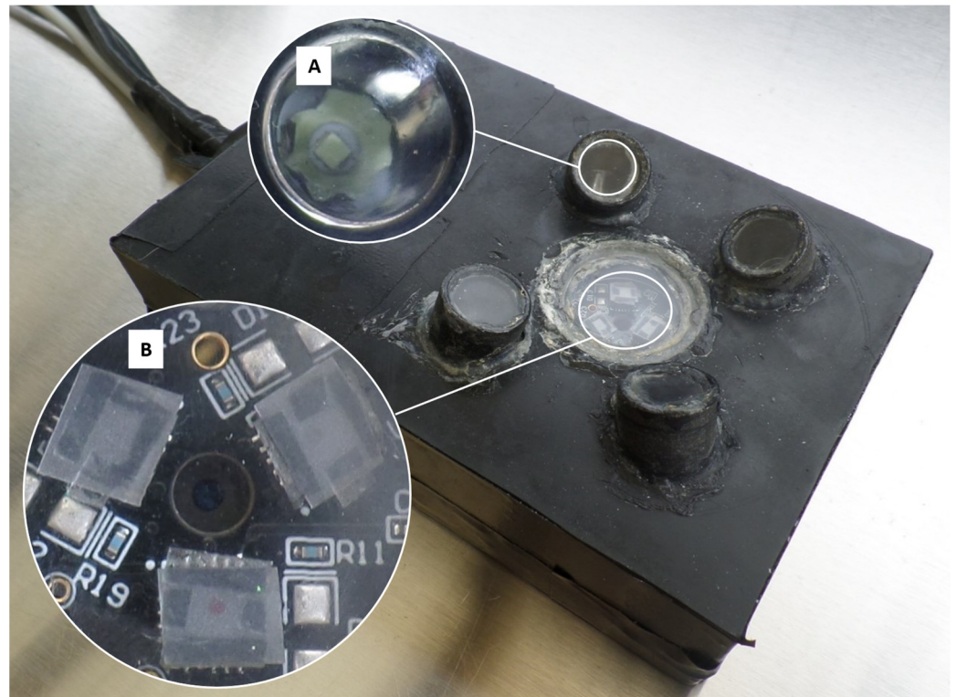
Figure 1. The HDPE waterproof housing (95 × 142 mm) with glued in clear acrylic windows. The four light tubes are arranged to focus the four light sources 75 mm beneath the sensors. (A) A SFH 4737 LED surrounded by a parabolic reflector; (B) the three AS7265x chips covered with Tsujiden D121UP diffraction film with the camera lens visible through the centre hole.
