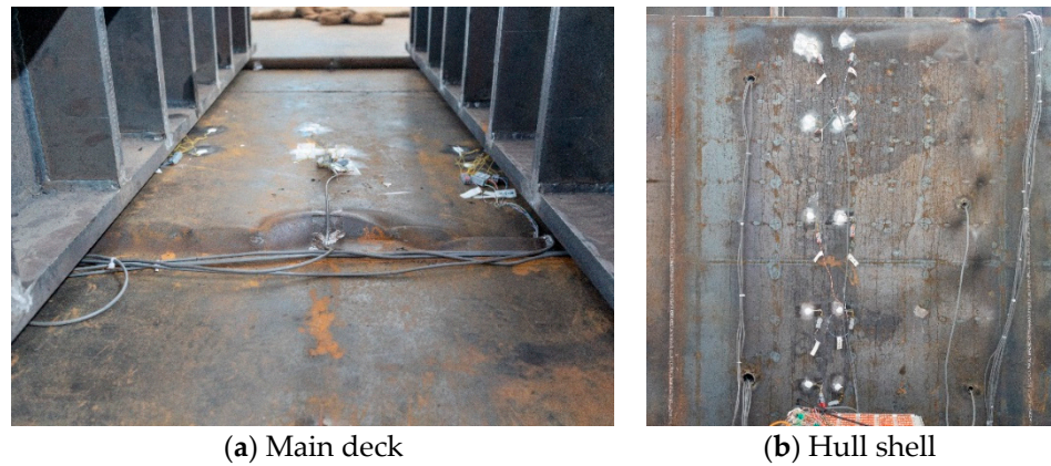
Figure 7. Collapse situation obtained by the collapse model test.
