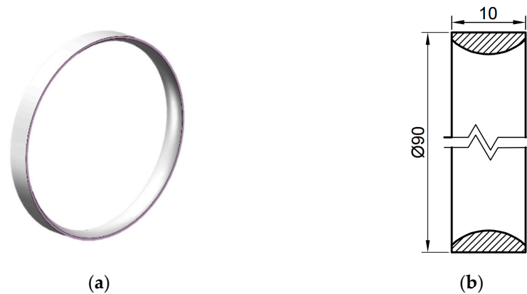
Figure 9. Outline drawings of reinforced rib section after processing: (a) 3D schematic diagram of strengthening ribs; (b) 2D schematic diagram of strengthening ribs.
