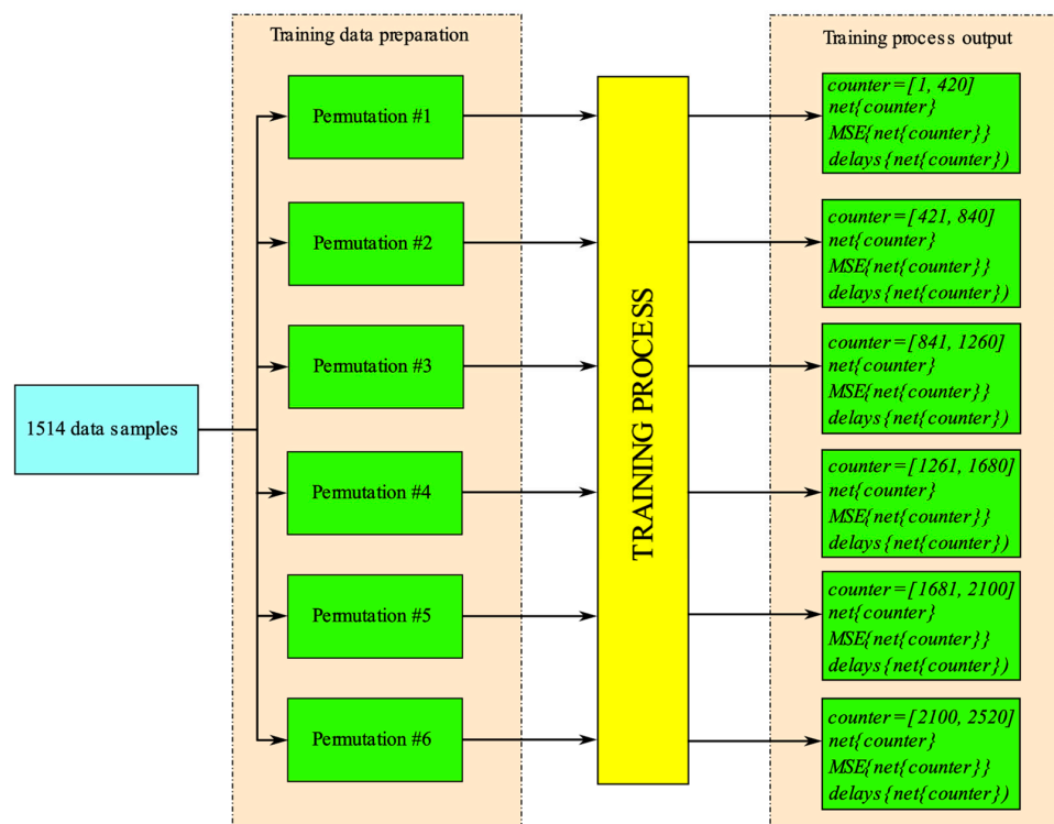
Figure 4. Flowchart of the data preparation methodology and training of the ANN NARX models.
